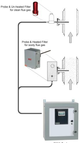
7200 Series Flue Gas Analyzer
